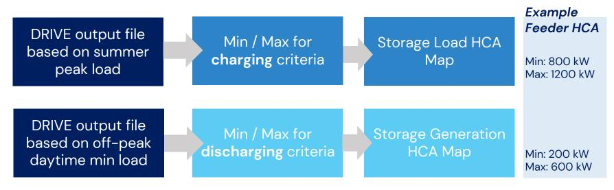
Note: The min/max generation criteria is specific to storage and not solar PV. This includes changes in fault current contribution and potential voltage changes.
