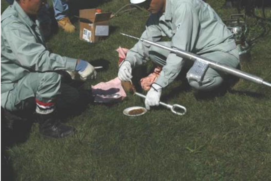
Figure 6-47 Application of high-temperature grease on core-grip portion
