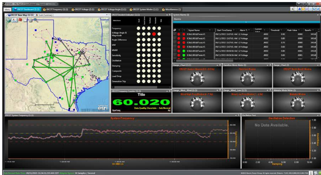
Figure 6-41 Visualization of wide area phase angles using RTDMS (ERCOT)
