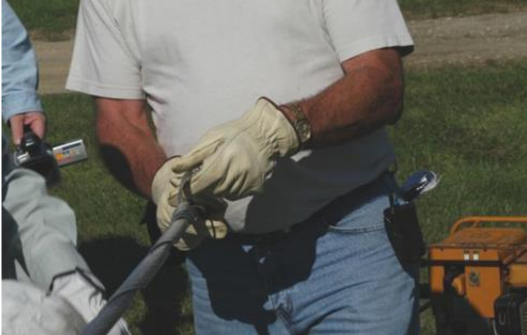
Figure 6-46 Removal of gap conductor strands at the termination at the EPRI Lenox Lab
