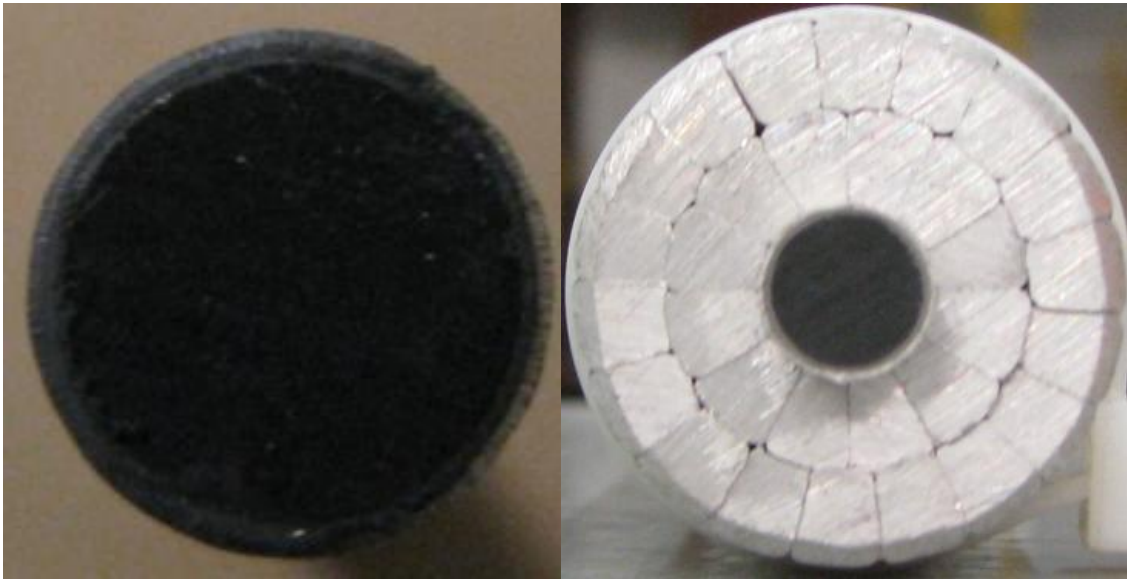
Figure 6-55 Cross-sectional views of Nexans cable—core (left), entire conductor (right)
