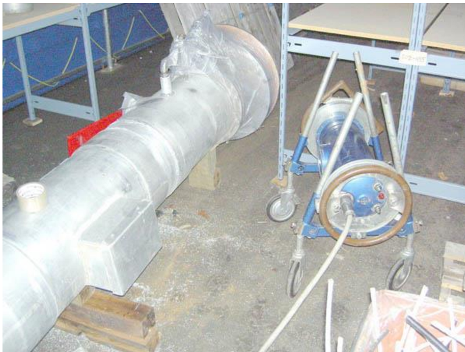
Figure 6-92 An example of a digital X-ray system deployed. The radiation source is the blue cylinder to the right. The digital X-ray plate is the red target to the left.
