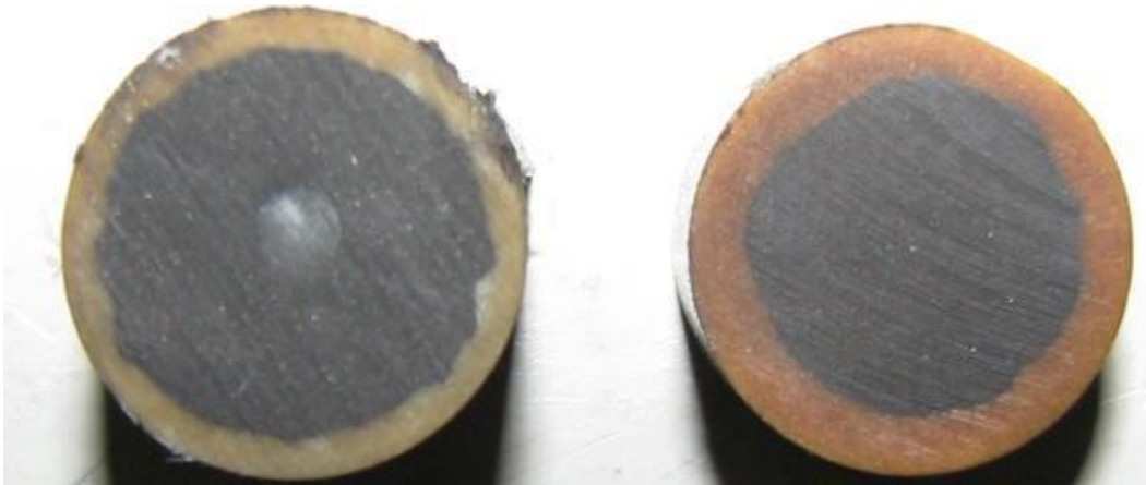
Figure 6-54 Cross-sectional views of mercury cable (left) and CTC (right) composite cores
