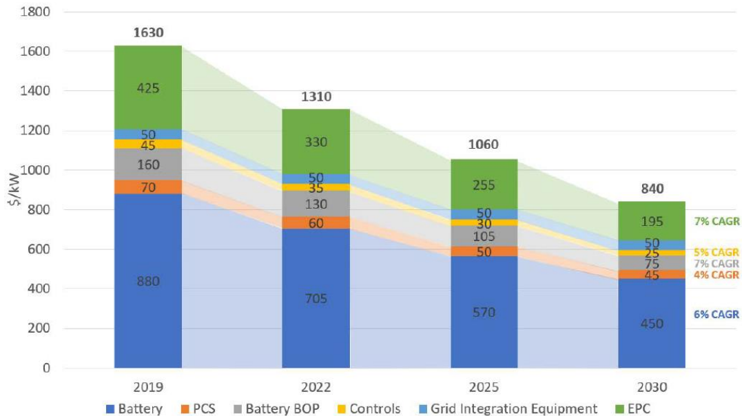
Figure 6-37 Installed costs projections for a 20MW, 4hr lithium ion system, 2019-2030. Source: EPRI
