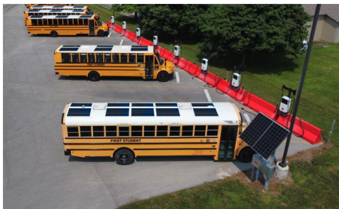
Figure 15: First Student Electric School Buses Featuring Rooftop Solar Panels at a Charging Depot
