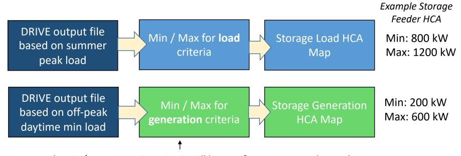
Note: The min/max generation criteria will be specific to storage and not solar PV. This includes changes in fault current contribution and potential voltage changes.
